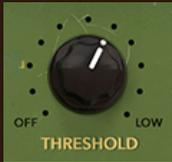
**THRESHOLD** From 0dBu to -50dBu, turning this knob clockwise lowers the point at which the compressor engages. Turning this knob FULLY counterclockwise disables the compression circuit entirely, but retains the input/output circuitry. This turns AR-1 into a very capable dirtbox with some of the loveliest distortion on the planet.
