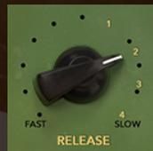
**RELEASE** Fully variable release ranges from 50ms (which is exponentially faster than the original) up to 2000ms. Clicking directly on Releases #1-4 will emulate the most popular timings of the hardware.
