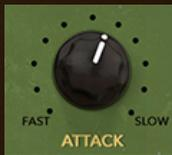
**ATTACK** Fully variable attack speed ranges from 1ms (which is considerably faster than the original hardware) up to 50ms.
