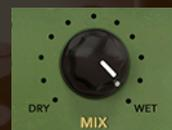
**MIX** Standard-issue mix knob adjusts the ratio of wet/dry signal for all your parallel compression needs.
