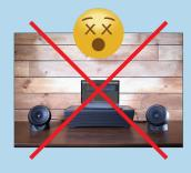
**DO NOT** place laptops or other electronics that are magnetically sensitive directly on the bass unit.
